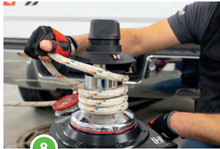
8 Pull rope through to take up any slack, then pass the rope on the stripper arm by winding rope clockwise and pulling tight to engage.
