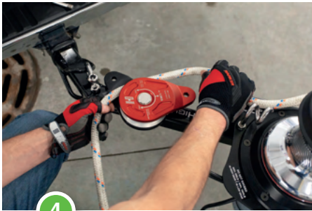
4 Lead rope through pulley: swivel plate open and put rope on sheave.
