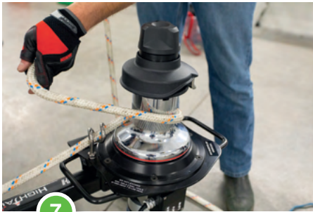
7 Start at the base of the winch and wind the rope in a clockwise direction. Ensure that the rope does not override on winch.
