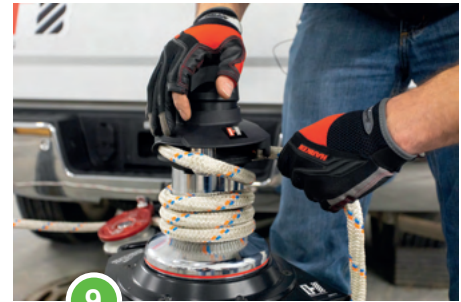
9 Insert the rope into the rope grab. Raise the cover for ease.
