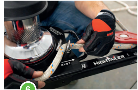
6 Feed rope through line drive.
